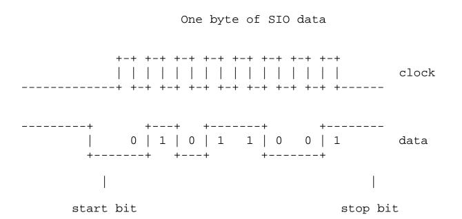
The SIO interface is used much like the resident disk handler. In fact, it uses the same device control block as the resident disk handler. After the control block parameters are set, a JSR is made to the SIO entry vector, SIOV, at \$E459 (58457).
